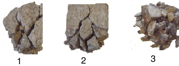
Fig. 4. Photos of natural stones samples after electric hydro-pulse processing.
