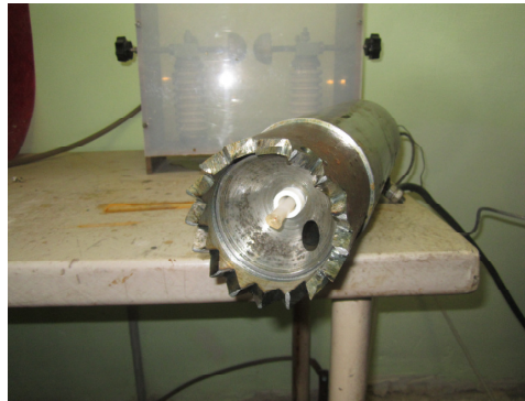
Fig. 2. The appearance of the electr-hydraulic drill
