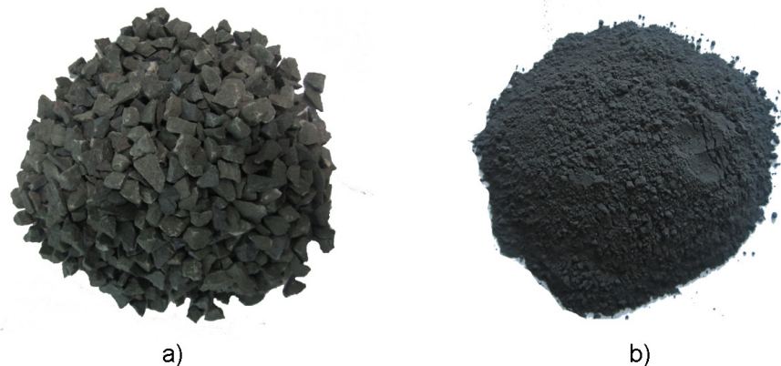
Figure 1. Various factions of crushed ore. I – original product before processing (fraction diameter of 5 \text{ mm} ), II – after electric pulse processing (fraction diameter of 0.2 \text{ mm} )
